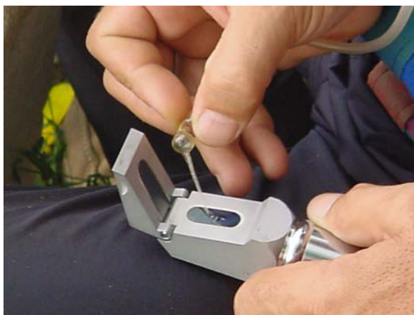
Figure 3. Determination of sugar concentration using a refractometer
